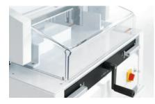
TRANSPARENT SAFETY GUARD A cut can only be executed, if the hinged, electronically secured safety guard on the front table is closed.
