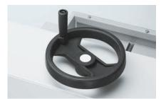
SPINDLE CLAMP WITH HAND WHEEL
