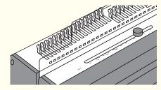
The precise settings required for different wire diameters can be set using a slider and scale positioned on the top side of the device. Switch formats quickly and easily by deselecting punching pins.
